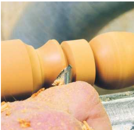
▲ Pic.22 When turning coves keep the tool handle tucked into your body. As you cut this shape make your body go through to the right as you slide the tool through the cut
